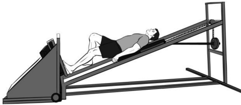
Fig. 1. The custom made inclined partial weight bearing sleigh used to perform the hopping task. Note the design whereby free weights are used to offset the weight of the sled seat.
