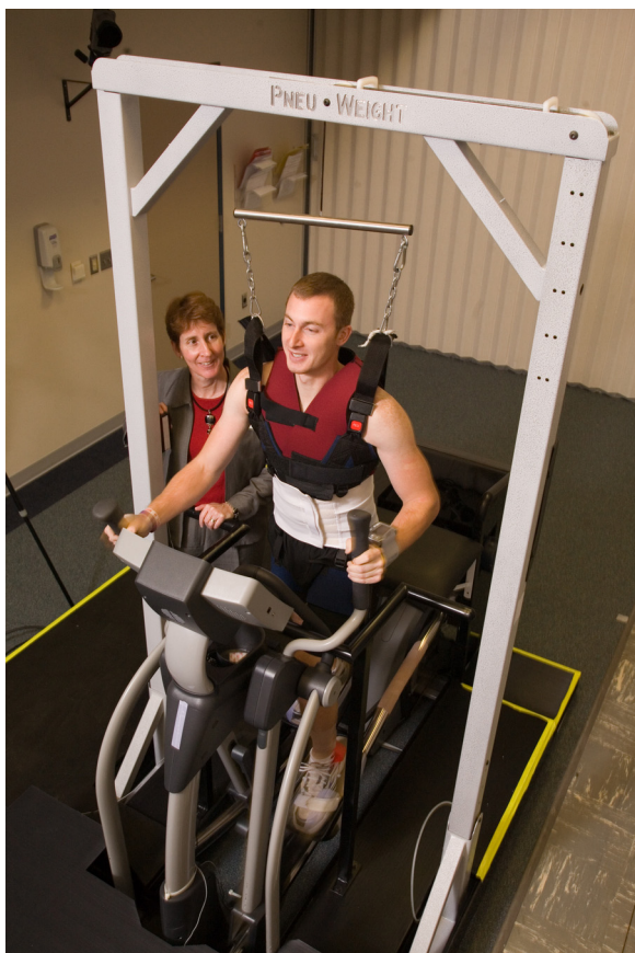
Fig. 1. Prototype motor-assisted elliptical trainer. An elliptical trainer was adapted to enable individuals with physical disabilities to improve walking and cardiovascular fitness. Stairs, ramps, support rails, pedal adaptations and a bench improved access to the device. An integrated sensor and motor system aided pedal movement and limb advancement. The system was integrated with a body weight support system.
