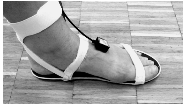
Fig. 1. Sensor configuration worn by a subject with inertial measurement unit (IMU) fixed on forefoot and pressure-insoles (reference system) beneath the foot.
