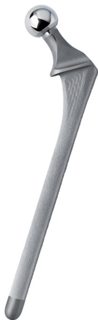
Fig. 1. Restoration HA stem. Stem fabricated of titanium alloy roughened by a chemical etching process. Hydroxyapatite is plasma sprayed over the entire length of the stem. Designed with a large proximal cross-section to provide for improved load distribution over a broad area. Distally, the design incorporates a cylindrical section to more effectively use the available bone of the diaphysis. The stem design incorporates a physiologic 127° neck-stem angle, neck length ranges, and a C-taper head to provide the surgeon with the ability to restore near-anatomical head position for proper leg length and biomechanical function.
