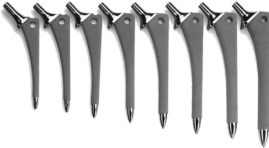
Fig. 1. The AML-plus stem. The series offers stem lengths in proportion to stem size in 1-mm increments and was introduced in Japan in 1997. The porous-coated area is 7/8 of the total stem surface with a 9/10 neck taper-trunnion.
