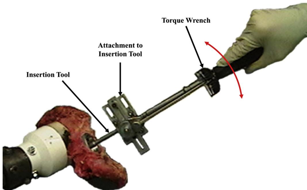
Fig. 1. A wrench was applied to the well-fixed, acetabular component through the insertion handle and tested to 60 in-lb (6.8 N-m) to test for gross stability of the component.
