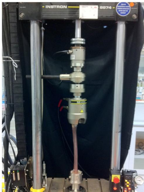
Fig. 3. The testing mechanism. The composite femur and stem are fitted in the Instron.
