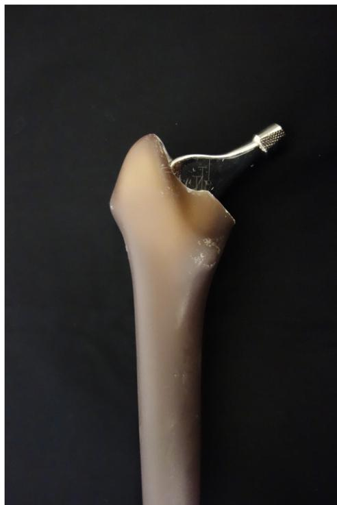
Fig. 2. Example of how a stem is fitted in the composite sawbone. The three markings on the stem can be used to determine the depth.
