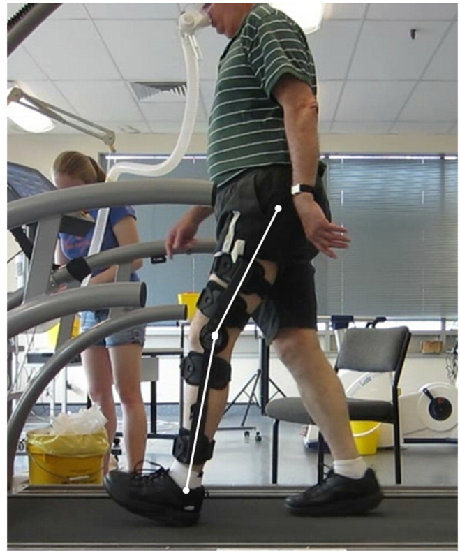
Fig. 1. A photograph illustrating testing set-up with gas collection apparatus applied to a participant walking on the treadmill during a 40^\circ brace restriction setting. The magnitude of the simulated FC is depicted.
