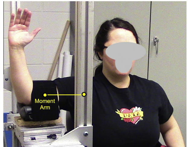
Fig. 1. Testing apparatus and participant arm posture for both testing sessions. Visual feedback was provided on the monitor situated in front of the participant (out of frame). Moment arm length (from the acromion to the centre of the rigid pad) was recorded for each individual to ensure proper positioning on both days, and to compute shoulder moments with the forces collected by the triaxial load cell.
