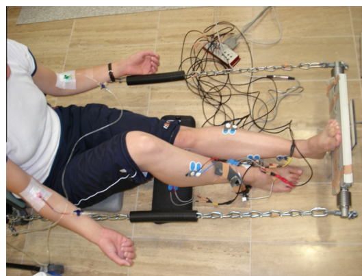
Fig. 2. Experimental setup. The subject is pressing with her left foot against the force transducer during a submaximal contraction. Intravenous catheters can be seen on both arms for blood sampling and tracer injection. Also visible are some of the SEMG electrodes connected to the acquisition device and an electronic goniometer around the right ankle.
