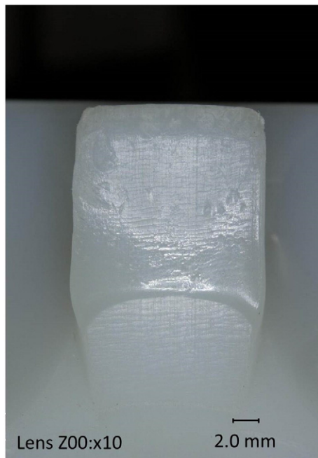
Fig. 1. Representative photo of an Optetrak® PS tibial post with “bowtie” damage.
