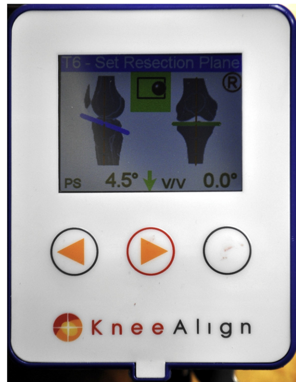
Fig. 2. The KneeAlign® navigation system display console.
