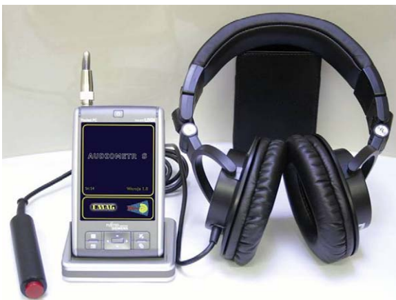
Fig. 1. The hardware used for the conventional and automated audiometry. The figure shows the Audiometer S PDA unit with a pair of ATH 50 headphones and the response button.
