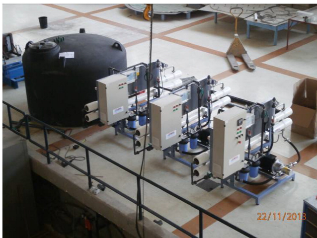
Fig. 2. Installed RO unit in the laboratory.
