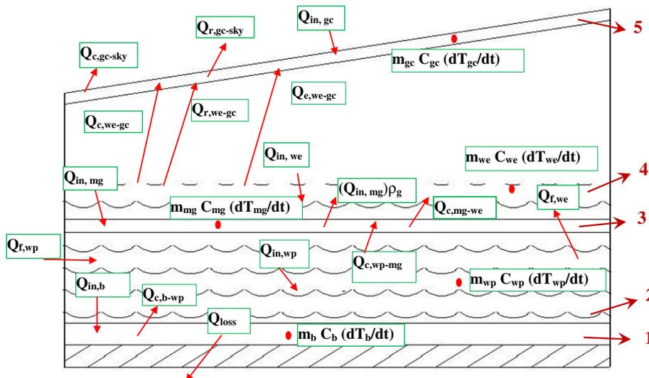
Fig. 1. Energy flow diagram of glass basin solar still. 1. Basin, 2. Water in preheater, 3. Middle glass cover, 4. Water in evaporator, 5. Glass cover.
