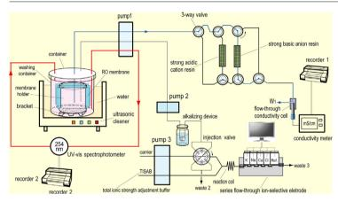
Sketch of a new ultrasonic-chemical cleaning system for researching cleaning effects of the waste reverse osmosis membranes with acids or alkali under ultrasound.
