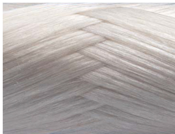
Fig. 1. Cross winding arrangement of the fiber.
