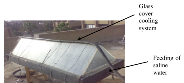
Fig. 1. The double slope solar still (passive solar still) with glass cover cooling.
