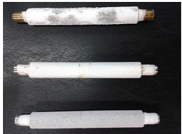
Fig. 3. Calcium carbonate fouling on different specimens.
