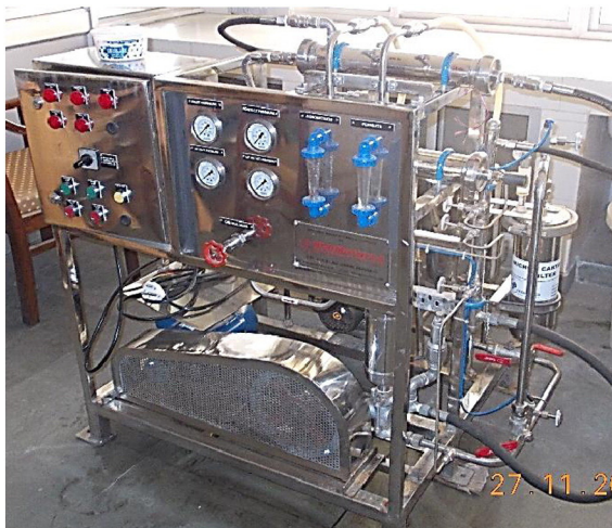
Fig. 2. Experimental setup with membrane filtration unit and PV system.
