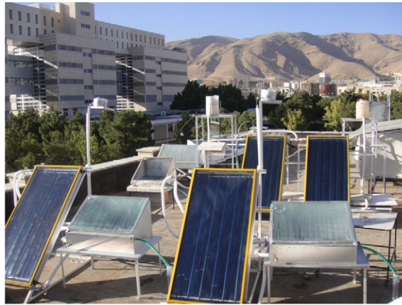
Fig. 1. (a) A schematic view of the active solar still system, and (b) a photo of the active solar still system.
