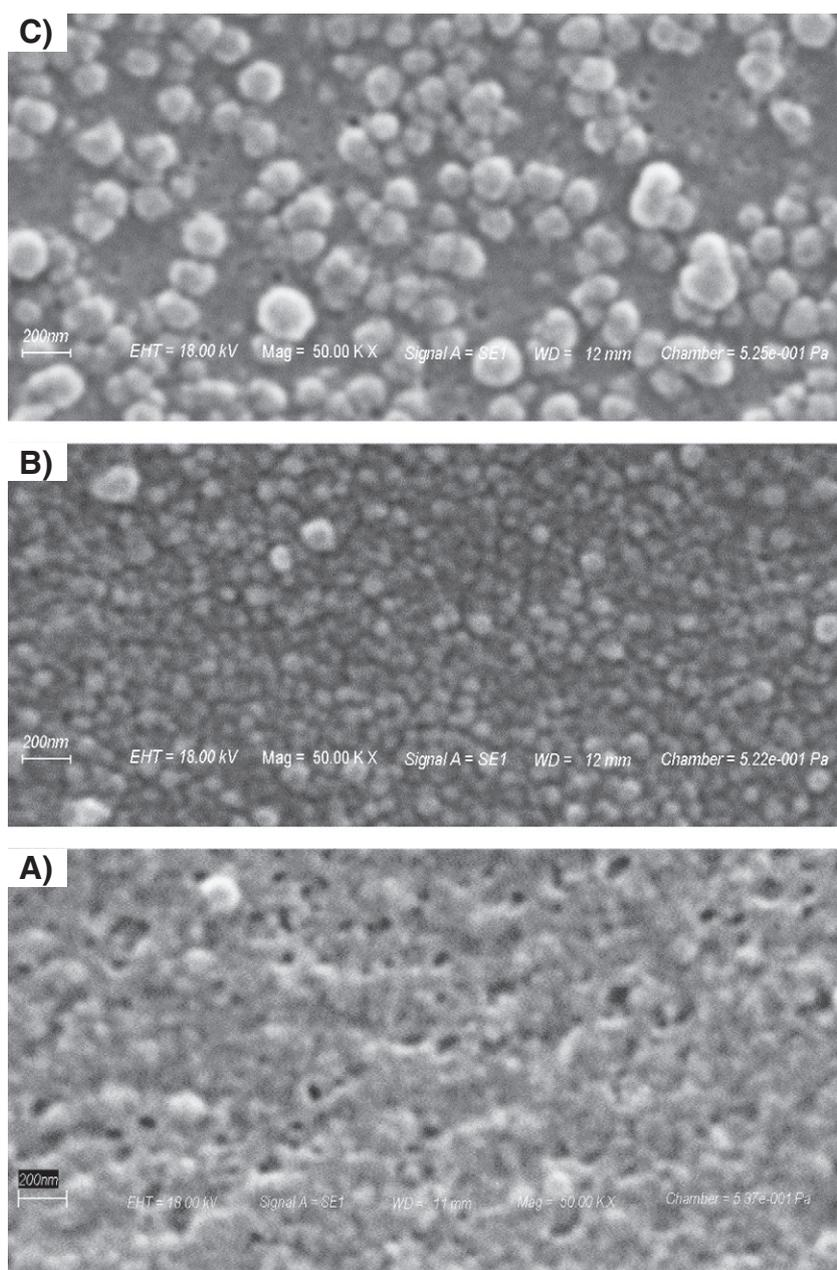
Fig. 1. Top surface SEM images of the TFC membranes, TFC-24 (A), TFC-15 (B) and TFC-12 (C).
