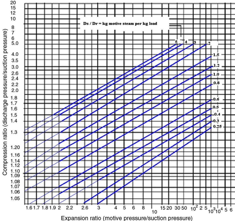
Fig. 2. Entrained ratio for different compression and expansion ratio [8].
