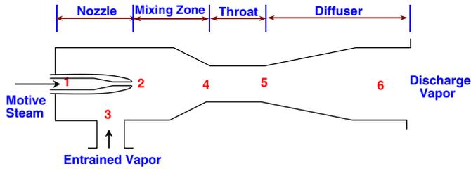
Fig. 1. Different processes in steam jet ejector.
