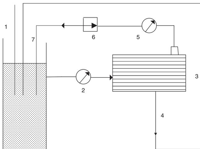
**Fig. 1.** Schematic diagram of the ultrafiltration unit: (1) feed solution, (2) manometer, (3) flat sheet module with PES membrane, (4) permeate stream, (5) manometer, (6) retentate rotameter, (7) retentate stream.
