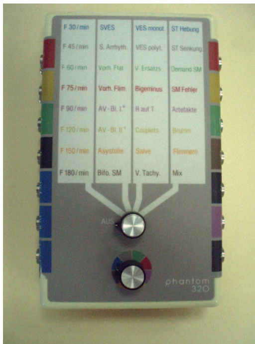
Fig. 1. ECG-simulator ("EKG-Phantom 320", Müller & Sebastiani Elektronik GmbH, Munich, Germany).
