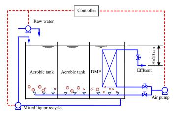
Fig. 1. Schematic diagram of the BDDM reactor process.
