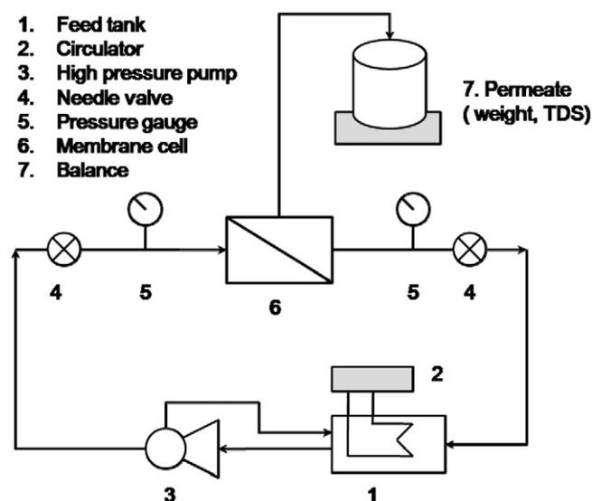
Fig. 1. Schematic drawing of a flat sheet membrane test apparatus.
