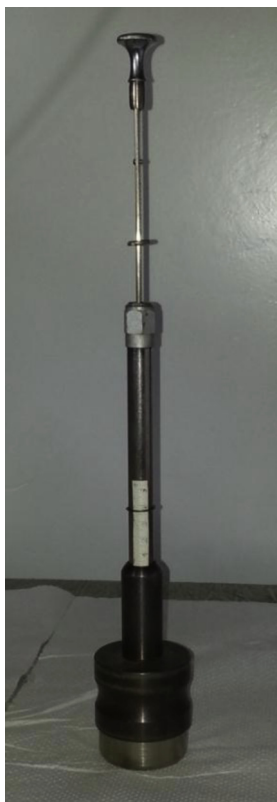
Fig 1. External view of the 1st device for measuring external pressure in transplanted kidney.
