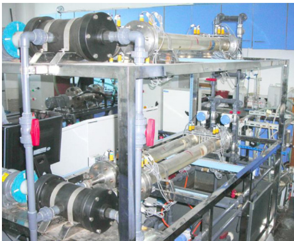
Fig. 2. Experimental setup of the parallel FS-ERDs.
