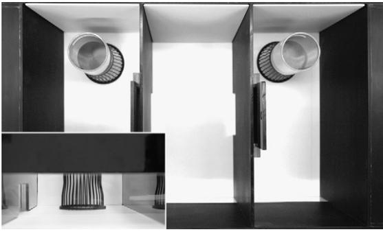
Fig. 1. Three-chamber social approach and social novelty arena. Three interconnected chambers are separated by two manually operated sliding doors. Outside compartments contain inverted wire cups to house a stimulus mouse. A steel weight and a clear Plexiglas cylinder are placed on top of the inverted cups to prevent lifting or climbing on top. The inset shows a front view demonstrating the clear Plexiglas window on the front of the arena which permits videotaping of the dyadic interactions of the mice.
