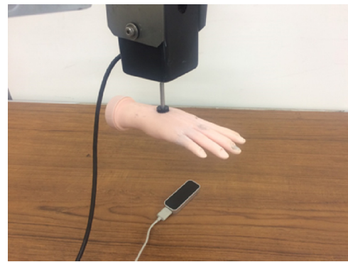
Fig. 1. Hardware system performance testing setup. A plastic hand model was attached to an electromechanical vibrator. The movement of the fingers was captured by Leap Motion below the hand and an accelerometer attached to the junction of the plastic hand and the vibrator simultaneously.
