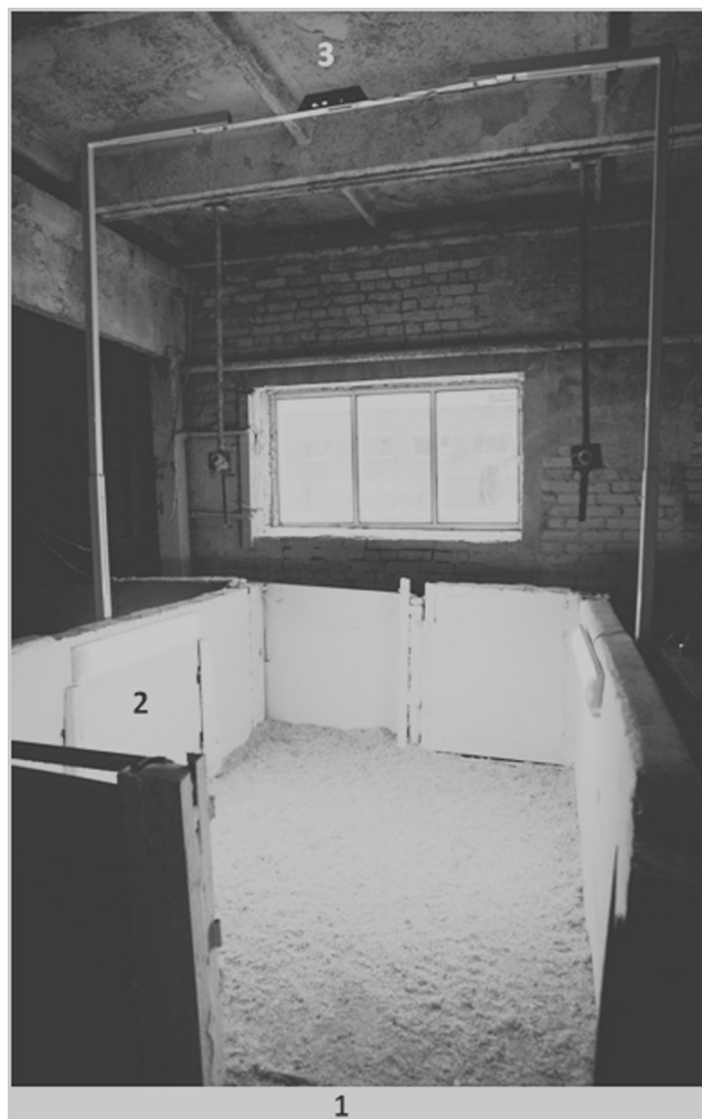
Fig. 1. The open field apparatus: 1 – arena (pen), 2 – halogen lamp, 3 – Kinect camera on the mount.
