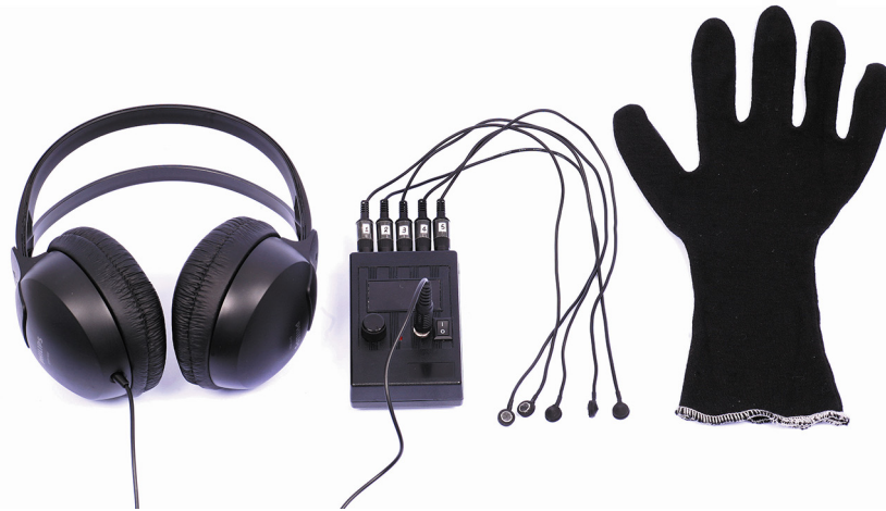
Fig. 1. Sensor glove components: earphones, amplifier, microphones, glove.
