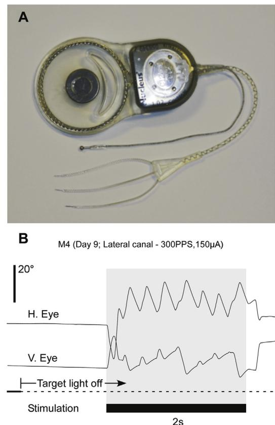
**Fig. 1.** The implantable portion of a multichannel vestibular neurostimulator based on a modified cochlear implant with a trifurcated lead for implantation into the three semicircular canals (A) and electrically evoked eye movement position traces (B). Eye position is plotted such that a negative value indicates a leftward eye movement for horizontal (H. Eye) and a downward eye movement for vertical (V. Eye) eye position traces.
