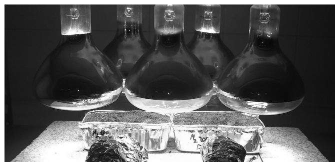
Fig. 1. Controlled burning of soil samples in aluminium trays by using infrared lamps.
