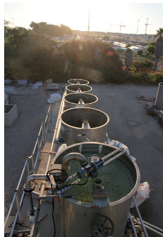
Figure 2. MBBR houses the bacteria where it is concentrated and protected.
