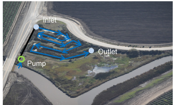
Fig. 1. Molera experimental wetland. This aerial photograph shows the sinuous wetland channel winding back and forth.
