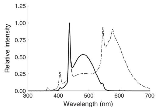
Fig. 1. Relative intensity of light sources with (solid line) or without a blue filter (broken line). The intensities were standardized at 435 nm.
