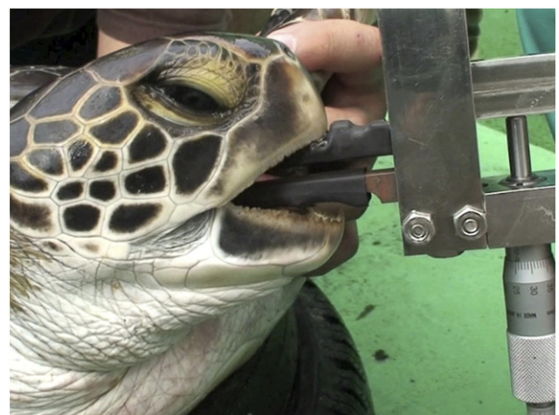
Fig. 1. An adult green turtle biting on the bite force apparatus.
