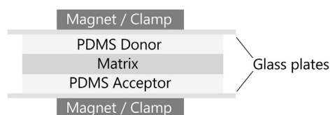
Fig. 1. Experimental setup with the glass plates and the assembly in between pressed together by magnets or metal clamps.
