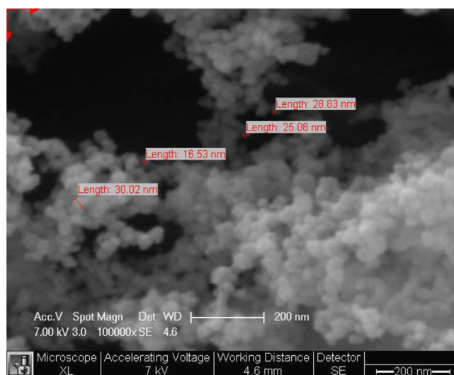
Fig. 1. ESEM image of nano-TiO 2 used in batch tests.
