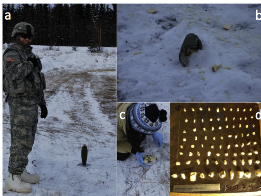
Fig. 1. (a) Set up for low order detonations of a 60-mm mortar; (b) the low order detonation; (c) collecting the pieces and (d) photograph of a subset of the massed pieces collected.
