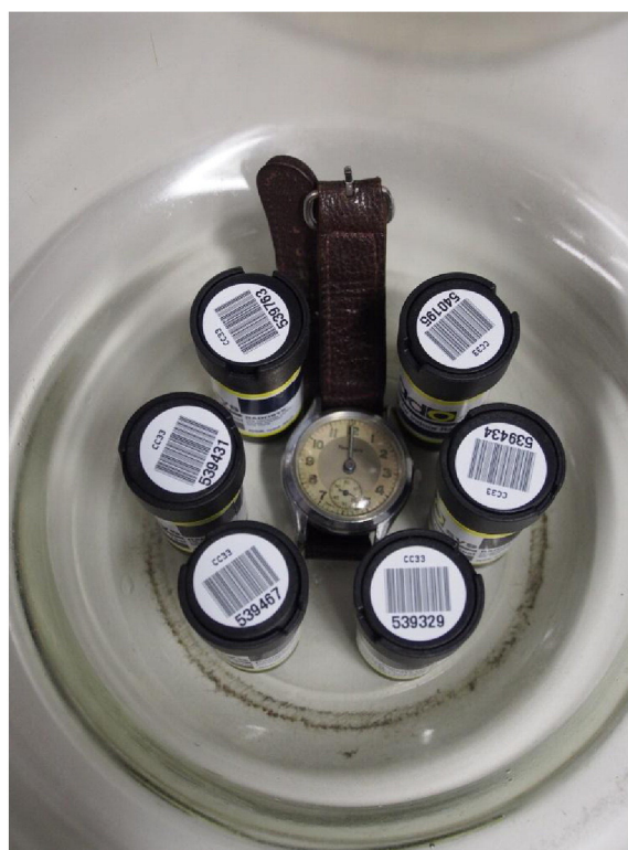
Fig. 1. Glass desiccation chamber adapted for radon and watch experiment. The join and plug were sealed using vacuum grease. SSNTDs were spaced as evenly as possible around the watch being tested.
