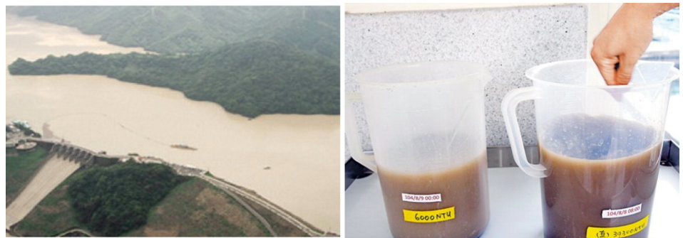
High turbidity water: (left) in a reservoir; (right) raw water in a water treatment plant.
