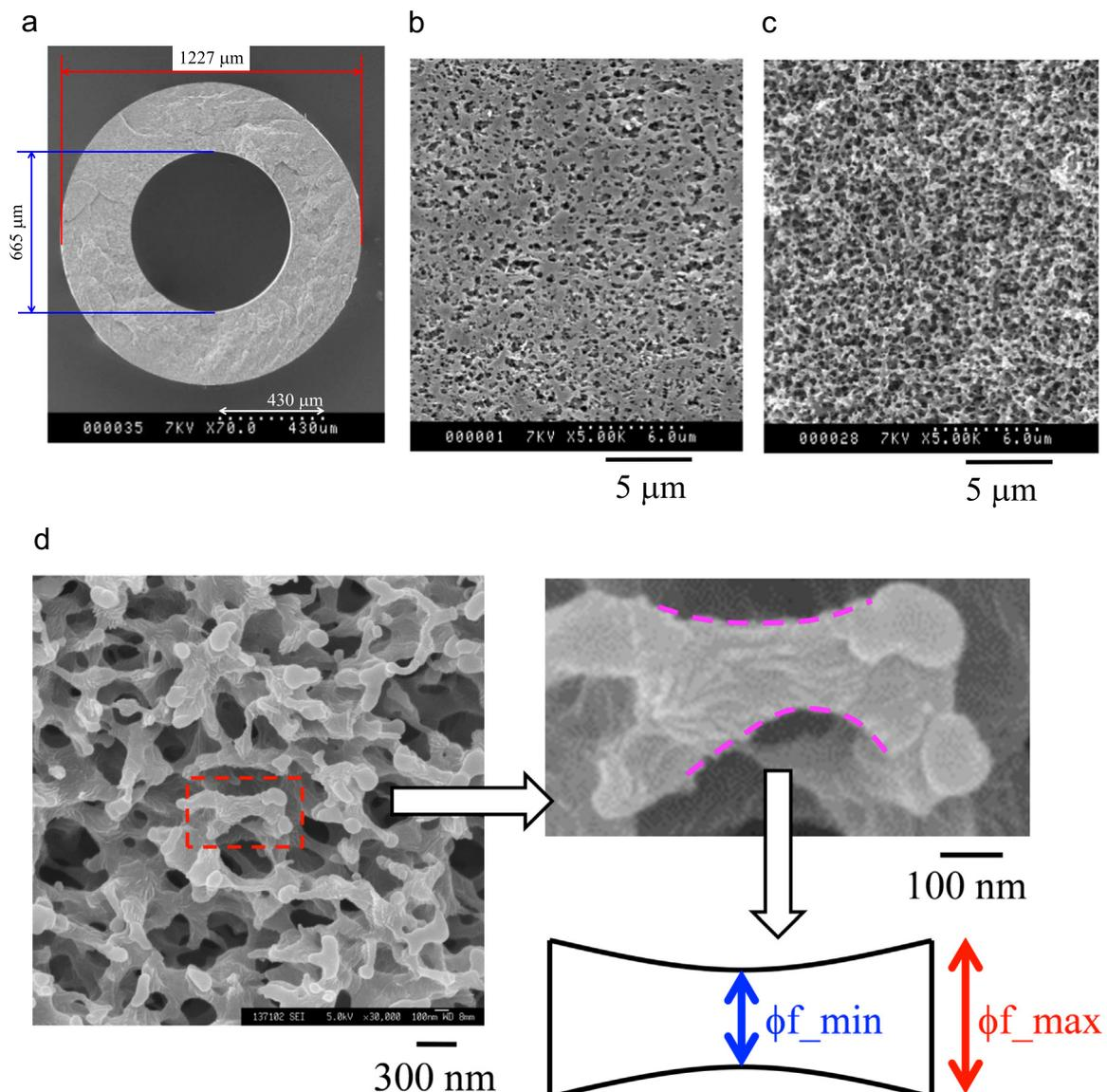
**Fig. 1.** Configuration and microstructure of the hollow-fiber membrane; (a) macroscopic view of cross section, (b) outer surface, (c) cross section, and (d) magnified view of (c).
