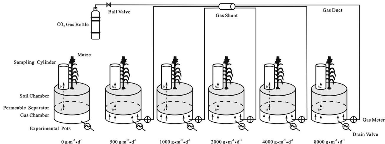
Fig. 1. Design of pot experiment for simulation of  $CO_2$  leakage. The  $CO_2$  injection flux was controlled at six different values; (a) experimental pots, (b) sampling cylinder.
