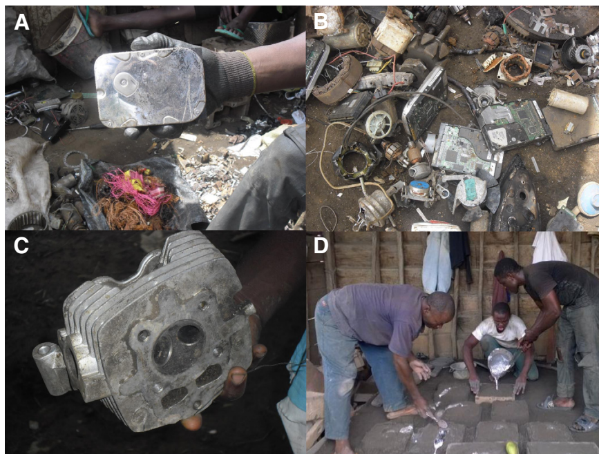
Fig. 1. Some source materials used in the manufacture of artisanal aluminum cookware in Cameroon. (A) Computer hard drive cover; (B) mixed scrap including computer parts; (C) motor bike engine part; and (D) molten scrap being poured into molds for pots.
