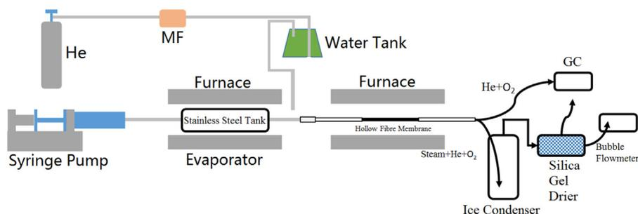
Fig. 1. Schematic of oxygen production using LSCF hollow fibre membrane.
