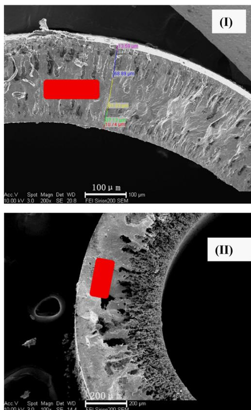
Fig. 2. Cross-sectional SEM images of two typical LSCF hollow fibre membranes spun using H<sub>2</sub>O as the internal and external coagulants. (For interpretation of the references to colour in this figure, the reader is referred to the web version of this article.)
