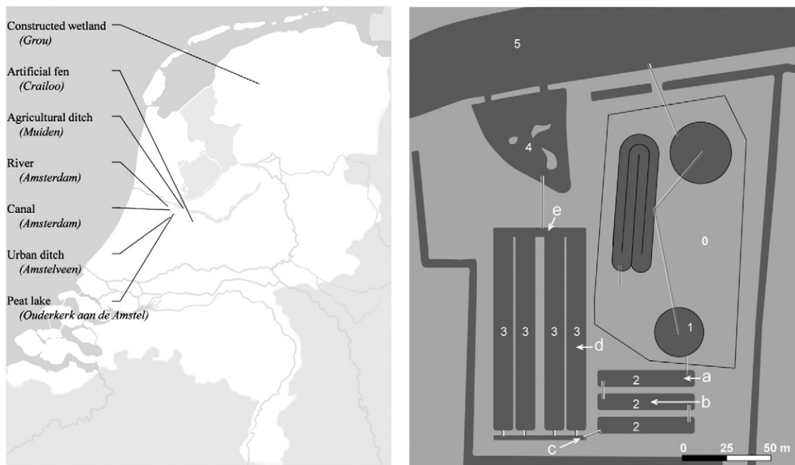
Fig. 1. Left: Sampling locations in the Netherlands. Right: Map of the WWTP in Grou, the Netherlands (0) with a sedimentation tank (1) which discharges treated municipal wastewater into a CW consisting of unvegetated ponds (2), reed beds (3) and an ecological buffer zone (4) which is in open connection the receiving channel (5). Sampling points were located at: PONDS-IN (a), PONDS (b), PONDS-OUT (c), REED-BEDS (d), and REED-BEDS-OUT (e).
