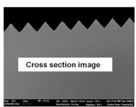
$\textbf{Fig. 1.} \ \ \textbf{Shape and dimensions of the prism-patterned master mold.}$
